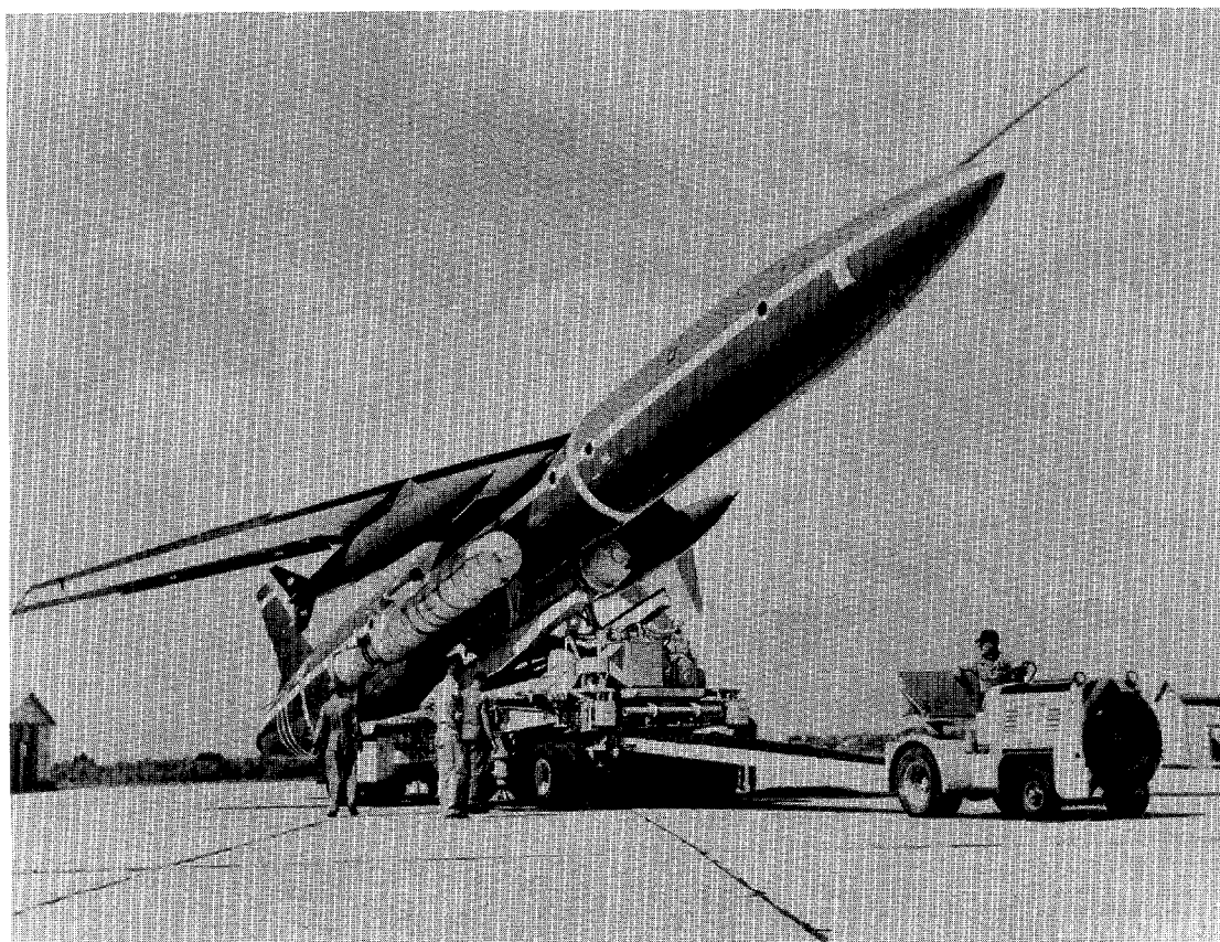
A Snark missile shown on its mobile launcher. The white canisters attached to both sides of the fuselage are solid-fuel rocket boosters.
