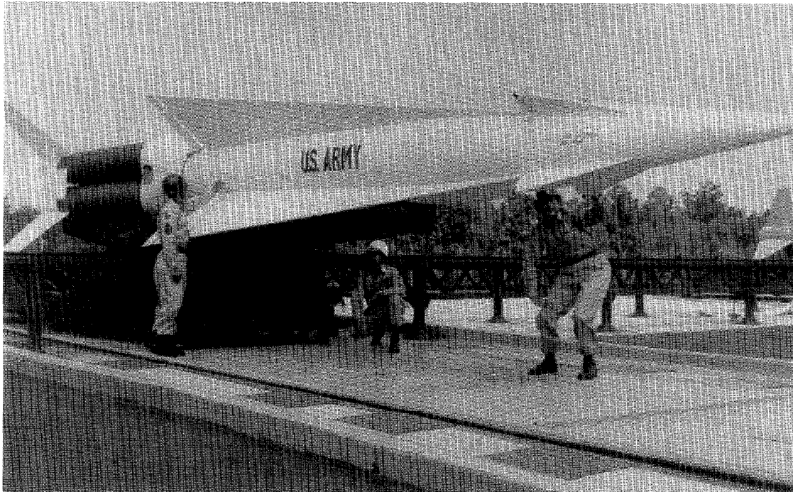
A solid-fuel Nike Hercules missile rests on its elevator-mounted launcher. The four dark colored solid-fuel boosters are clustered together just forward of the tail.
