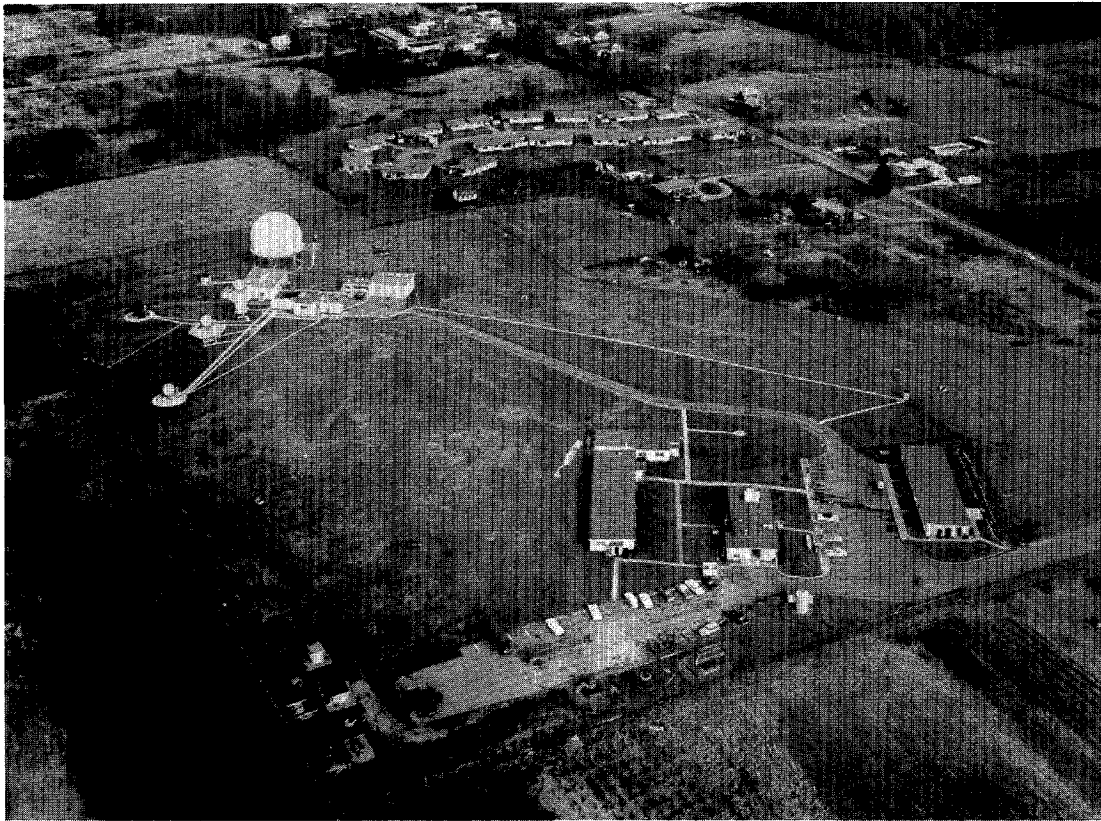
An aerial view of the integrated fire control area, Site S-61, Vashion Island, Washington. Although this 1971 photograph shows the site configured to handle the Nike Hercules, all of the earlier Nike Ajax radars are still in place. Positioned outward from the radar dome are the target-ranging radar, target-tracking radar, the missile-tracking radar, and at the forward edge of the installation, the low-power acquisition radar. The buildings in the foreground are barracks and support buildings.
