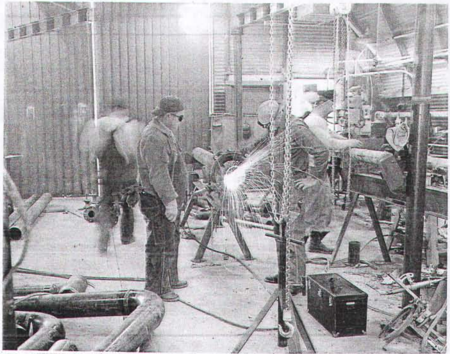
W22. Two views of Crouse oxygen-acetylene beveling machine in operation at the flanged pipe shop.
