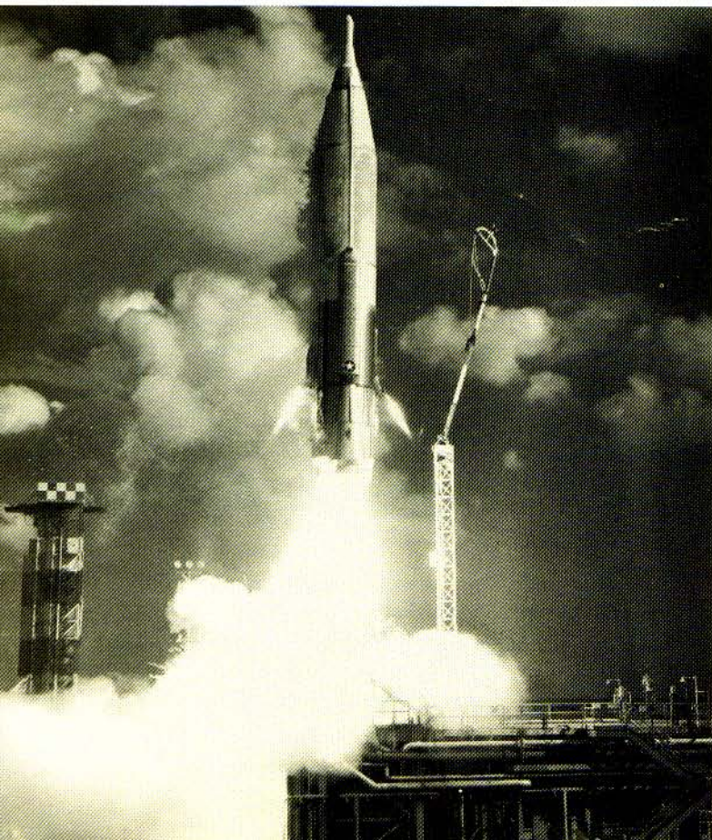
Below, a remote camera near the launch pad catches this Atlas with its three engines and two vernier engines on the sides spouting flame.
