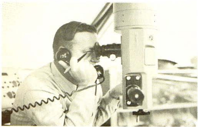
A missileman gets an accurate reading with his periscope that extends through the cement roof of an ICBM blockhouse.
